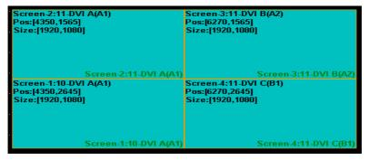
The default resolution and size of window for each output port is 1920\*1080 Select one output and right click, enter the screen property setting to set parameters of each output.
