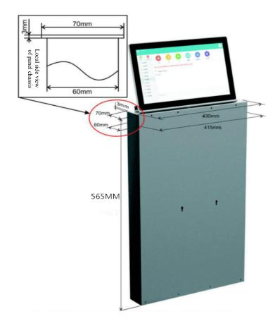
Notes: before installation, please unscrew the two "fixation screws for transportation" on the covers and the fixing clip of side display and clean up the foam filler in the flip gate
