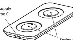
Spring probe: When the charging tray power on, expansion mic's charging copper ring contacts spring probe for charging
