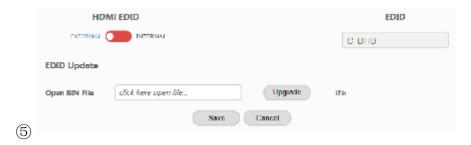
**HDMI EDID:** When set to Internal, the EDID communicated to the source is the one stored in the device's internal memory.
