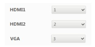
Sets the priority to use when the switch mode is set to priority mode. 1 is the highest priority and 3 is the lowest.
