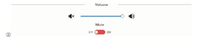
Volume control outputs for the amplifier and the audio extractor. Adjusting the slider to increase or decrease outputs for the amplifier and the audio extractor. Toggle is the Mute setting to silence the amplifier and the audio extractor outputs. Mute setting does not silence the audio on the HDMI output line.
