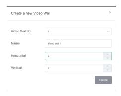
You can set the Video Wall ID, Name, Horizontal and Vertical panel numbers. Then click "Create" to create the Video Wall.
